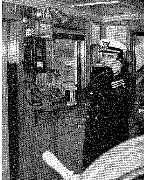
Captain Leo Moll of the John G. Munson used this type of radiotelephone set when he skippered the W. F. White. Later installations are alongside the pilot house lookout window for greater convenience.
